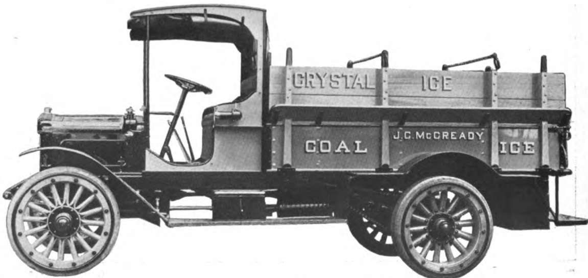
BROCKWAY MODEL "I" TWO-TON CHAIN DRIVE COAL TRUCK Manufactured by Brockway Motor Truck Co., Cortland, N. Y.
